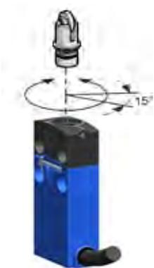
All actuators can be adjusted from 15° to 15° on 360° relative to the body
